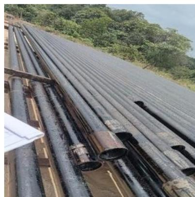
Gambar 8. Sambungan (Joint) Tubing J-55
